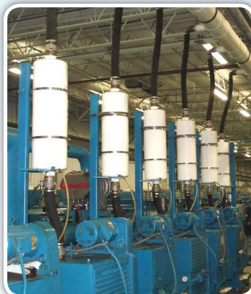
Edwards Vacuum Pump: Glass Coating Application Two-Stage Straight Through Discharge Oil Mist Eliminator
